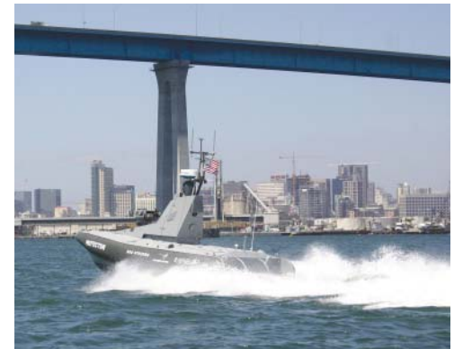
RHIB USV provides harbour surveillance using radar and EO together with interdiction weapons if required
