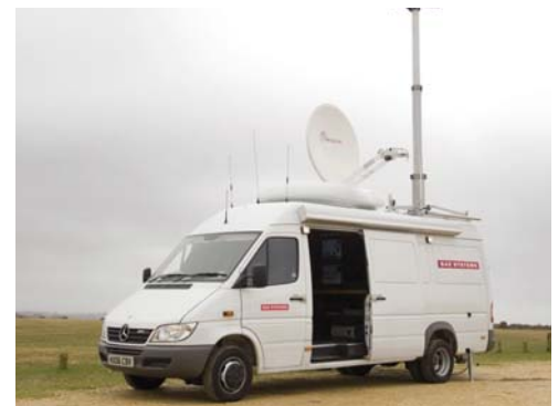
Deployable Surveillance Unit (DSU) deployed as UUV command station
