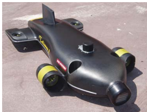
Talisman L - designed for two-man deployment from small craft
